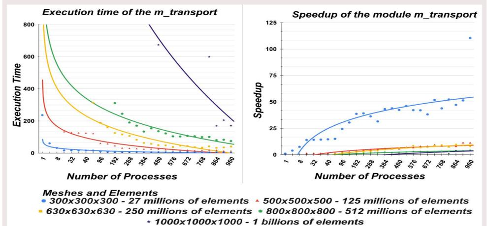
Figure 3: Speedup with an execution of 960 processes using 20 computational nodes of SDumont's Cascade Lake architecture
